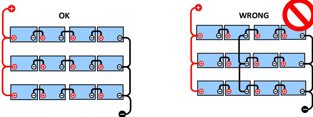
Due to the voltage drop over the positive and the negative cables the midpoint voltage are not identical.
